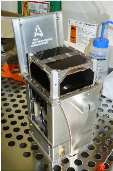
Figure 2: SwissCube FM in its SPL deployer
