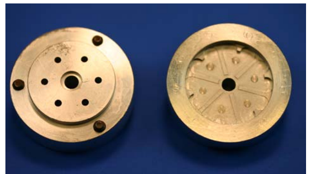
Figure 15 parts of the mould. Left : male part with surplus evacuations. Right : female part. Note the tops of the extraction screws confounded with the bottom of the mould.
