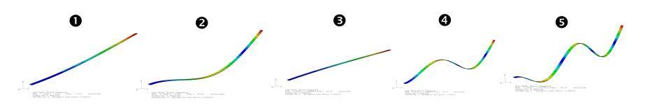
The frequencies at which the antennas could disturb the attitude control of the satellite are characterized
