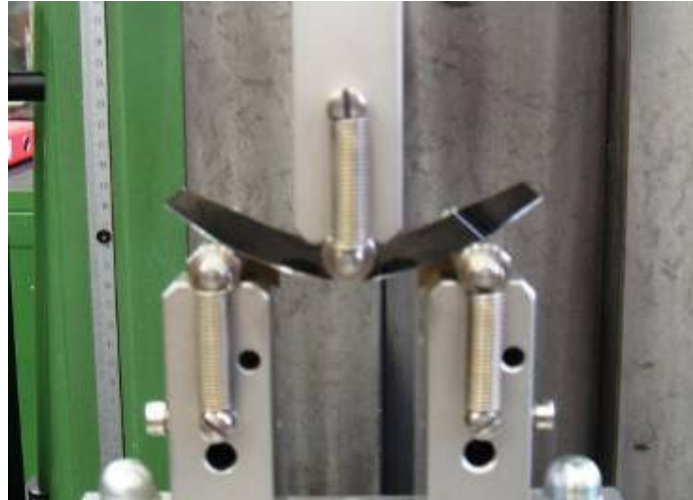
• Figure 80 Three points flexural test of a solar cell.
