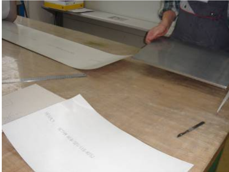
Figure 32 Preparation of the aluminum plate and cutting of plies.
