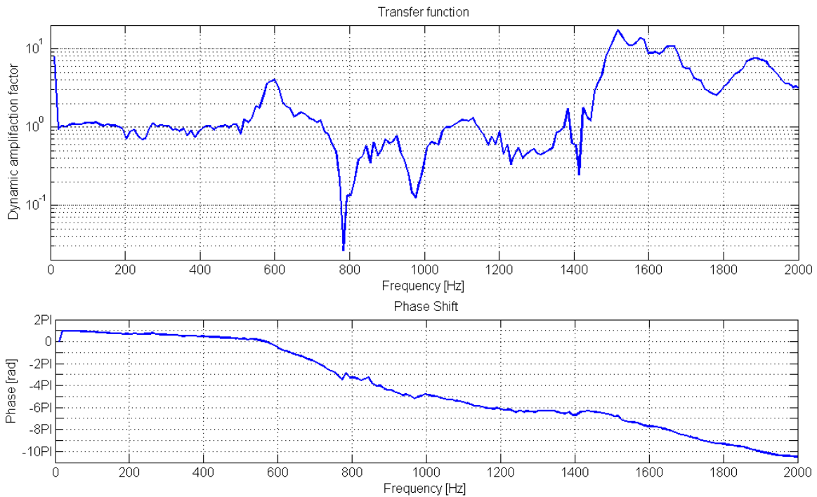
Figure 76 Random vibration in Y-axis, Transfer function and Phase shift for Accelerometer 3.
