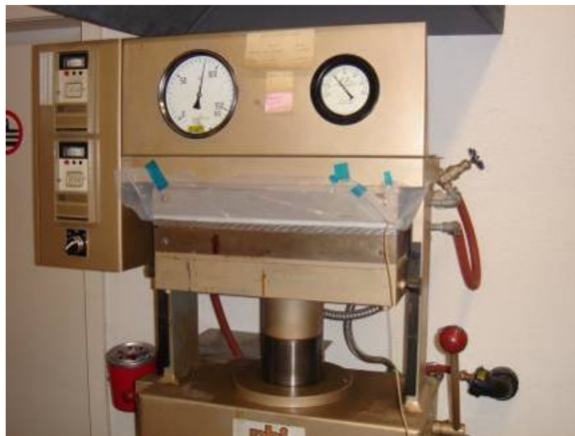
Figure 33 Hot press used for the manufacturing.
