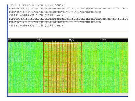
Another interesting point is the impact of the PA temperature on the transmission frequency. To measure this change, it has first been necessary to enable the PA, and therefore to generate a 1kHz signal with the microcontroller to set Vctrl equal to 2.6V. The measured frequency shift when the PA is turned on is around 400Hz.
