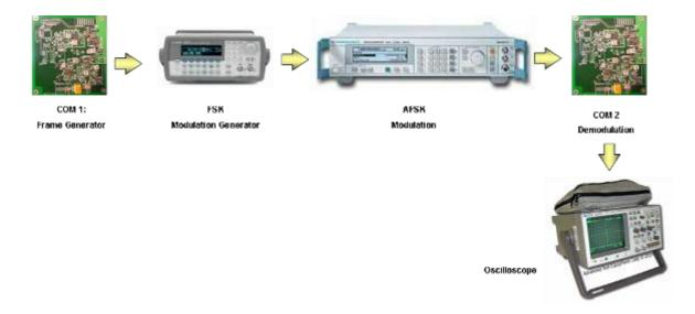
The frames demodulation at COM\_2 has been successfully done. Two signals have been used to confirm and valid the data reception: P5.2 gives a logical high when a frame is received (one frame is equivalent to 23 Bytes); P5.0 changes its state if the received frame was correct. This is shown in the next two figures:
