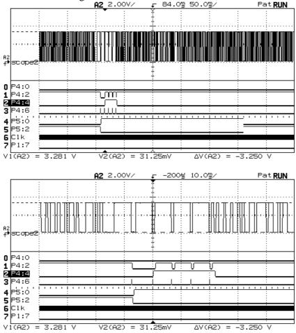
The A2 port is the demodulated signal at the COM's modem; P4.6 represents the flag reception and P4.2 and P4.4 indicate the reception mode:
