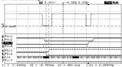
A simultaneous uplink and downlink communication test has been performed. The full duplex communication was also possible.
