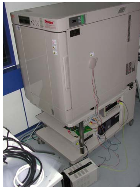
Figure 6 Temperature Chamber (Gyroscope is place inside the chamber) [photo from [R1]]
