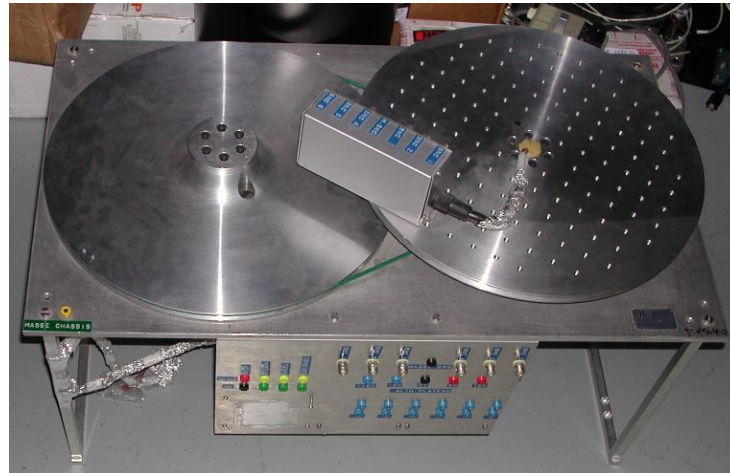
Figure 5 Rotational Table (Gyroscope is place on the right; fast mode in the picture) [photo from [R1]]
