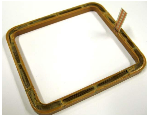
Figure 4-8 : Finished/moulded MT view. The small PCB prevents the break of the copper wires during the moulding and facilitates the soldering.
