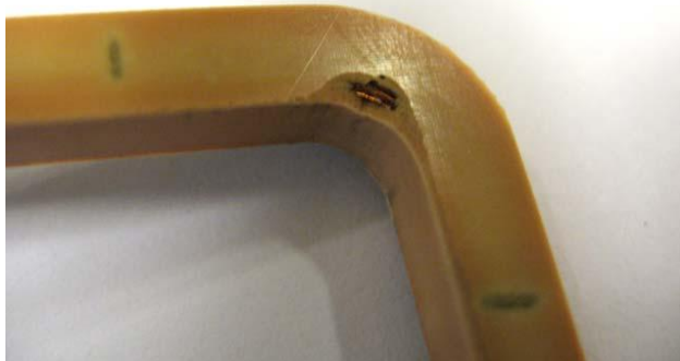
Figure 4-9 : MT detailed view. A break can be observed in the corner.
