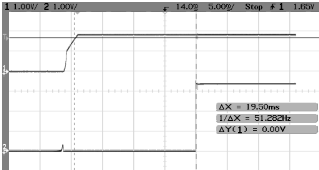
Figure 7-1 : power-on reset measurement
