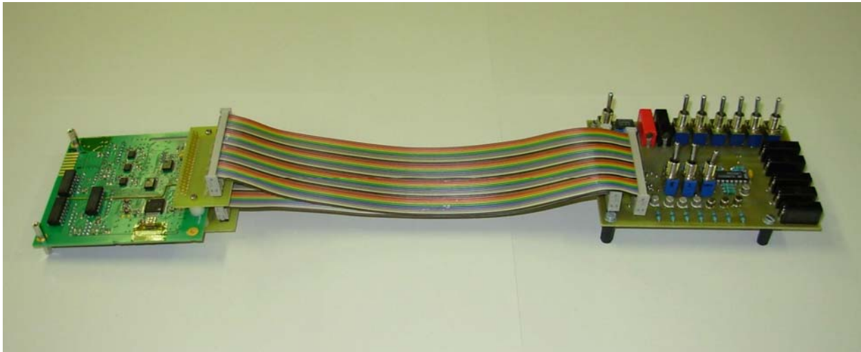
Figure 4-25 : PMB and testing board interconnection
