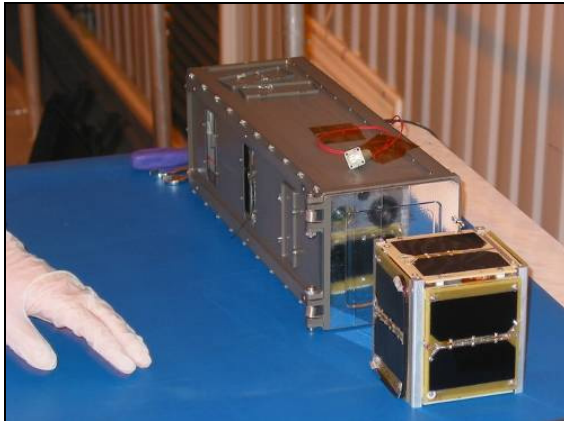
Figure 1-2 : Poly Picosatellite Orbital Deployer (P-POD)
