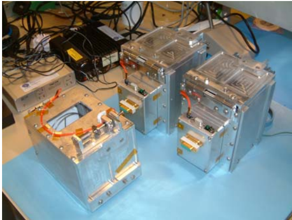
Figure III-10: T-POD's during integration of SSETI-Express.
