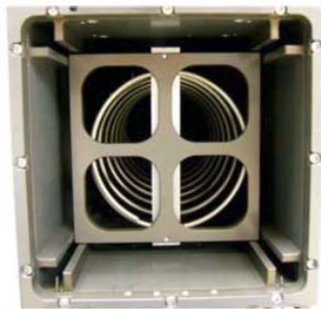
Figure 3 : Cross section of the P-POD.
